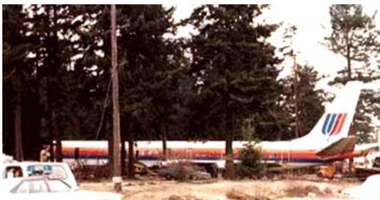
On December 28, 1978, a DC8 with 189 persons on board on final for Portland's airport lowered the gear. There was a loud bang and the plane yawed as a right main landing gear cylinder failed and enabled the gear to free fall into place. The force of the free fall destroyed the micro switch that indicates that the gear is down and locked, which it was. With no green indication light in the cockpit to verify that the gear was down, the Captain initiated a go-around and for the next hour and
